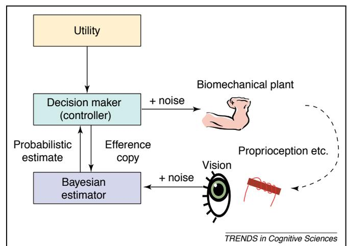
**Figure 3.** Optimal controllers. In generating a movement, the controller, an optimal decision maker, takes into account both the output of the Bayesian estimation process as well as the utility function. The Bayesian estimator combines inputs from the sensors (for example, about limb positions) with prior knowledge in addition to the efference copy – the signal sent by the CNS to the muscles.
